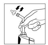
2. Twist the *OtoClear*® tip on the luer lock fitting of the adapter wand. (Be sure to tighten the *OtoClear*® tip securely).
