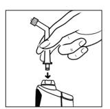
1. Push the adapter wand into the positioning wheel.
